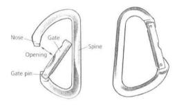
Fig. 34 - The parts of a carabiner.
