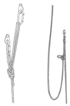
Fig. 284 - Y-belay on compact hangers and non-locking carabiners.
