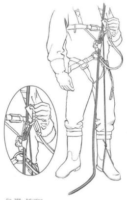
Fig. 388 - Adjusting the Mao system, or Italian footloop.
