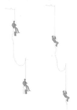
Fig. 42 - Sketch of situation during descent (left) and climb (right) before a main or rebelay anchor fails.
