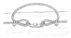
Fig. 100 - Anchor set along a wire cable traverse.
