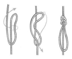
Fig. 68 - Directional eight (in-line figure eight).
