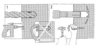
Fig. 80 - Setting an anchor with a power drill.
