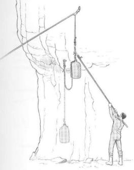
Fig. 46 - Installing a drop-test mechanism.
