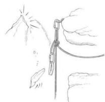
Fig. 244 - With this rigging, the anchor plate could break under the shock load following the failure of the backup anchor.
