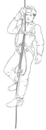
Fig. 191. - The double bungee system. The chest roller is mounted on a horizontal metal plate incorporated into the chest harness to minimize chest compression.
