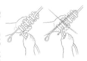
Fig. 153 - Left: Install the rope correctly by weaving it over the top bar and behind the first (already closed) notched bar. Right: Installing the rope backwards on a rack will cause the bars to pop off as soon as the rack is loaded, resulting in a free fall.
