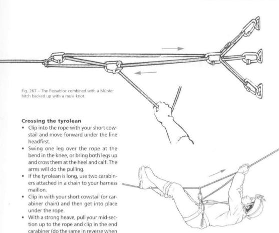
Fig. 268 - Travelling along the tyrolean.
