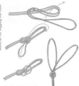
Fig. 56 - Double figure eight on a bight, or rabbit ear knot.
