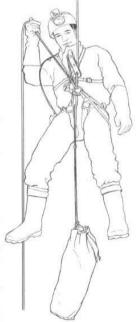
Fig. 149 - Use your right foot to keep the rope from tangling with a tethered pack.
