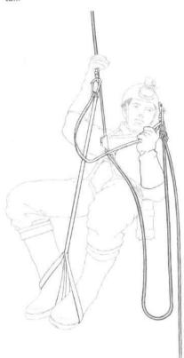
Fig. 166 - Slack appears in the cowstail as you start climbing; you can now remove it from the anchor plate.
