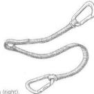
Fig. 18 – Double cowstails made from knotted dynamic rope (left) and sewn webbing (right).
