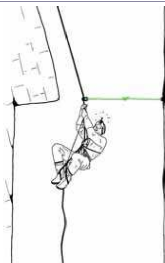
Correct position for a deviation
