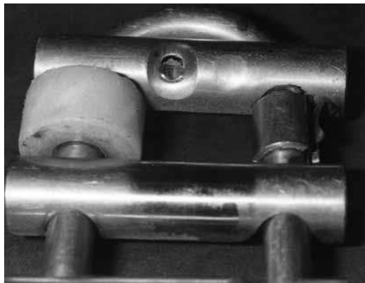
Rack spacer and worn hollow brake bar
