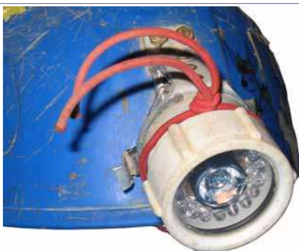
One of many prototypes. A single central 'Luxeon' for spotting surrounded by 18 x 5 mm LEDs for normal use. Each set of LEDs is separately powered and switched to provide redundancy
