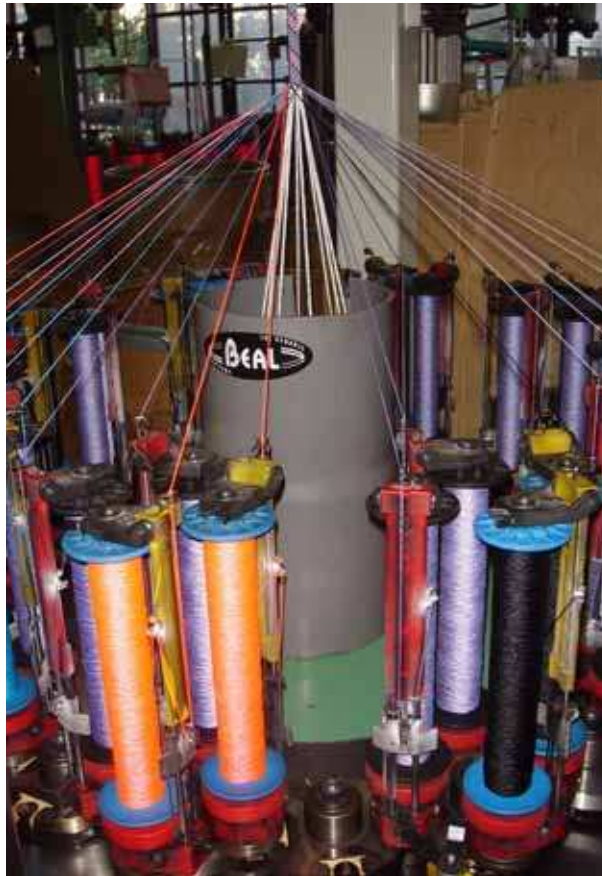
Kernmantle rope under construction (Beal factory/website)
